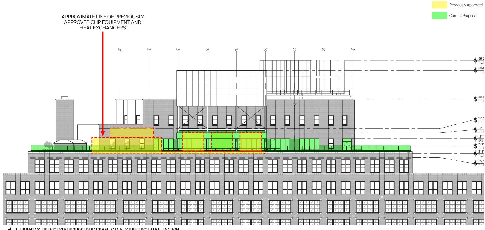
CURRENT VS. PREVIOUSLY PROPOSED DIAGRAM - CANAL STREET (SOUTH) ELEVATION NTS
